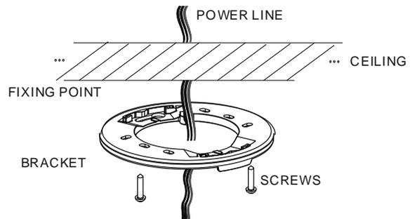
3. Connect mains supply to the luminaire.
