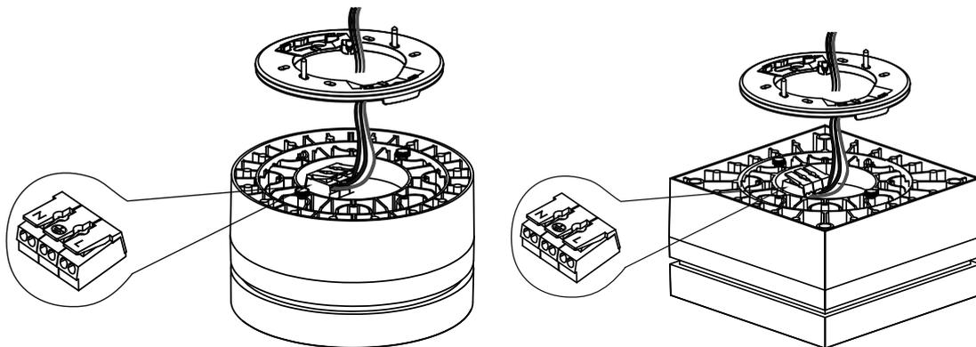
4. Place the luminaire onto the ceiling fixing and secure it
